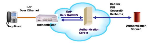
Figure 55: 802.1x and EAP network architecture
