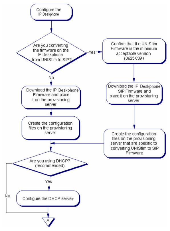
Figure 4: Installation of IP Deskphones with SIP Software, page 1 of 2
