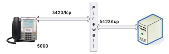
Figure 37: Connection reuse and a firewall
