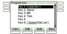
Figure 20: Main feature key programming screen showing Speed Dial List provisioned on key 6
